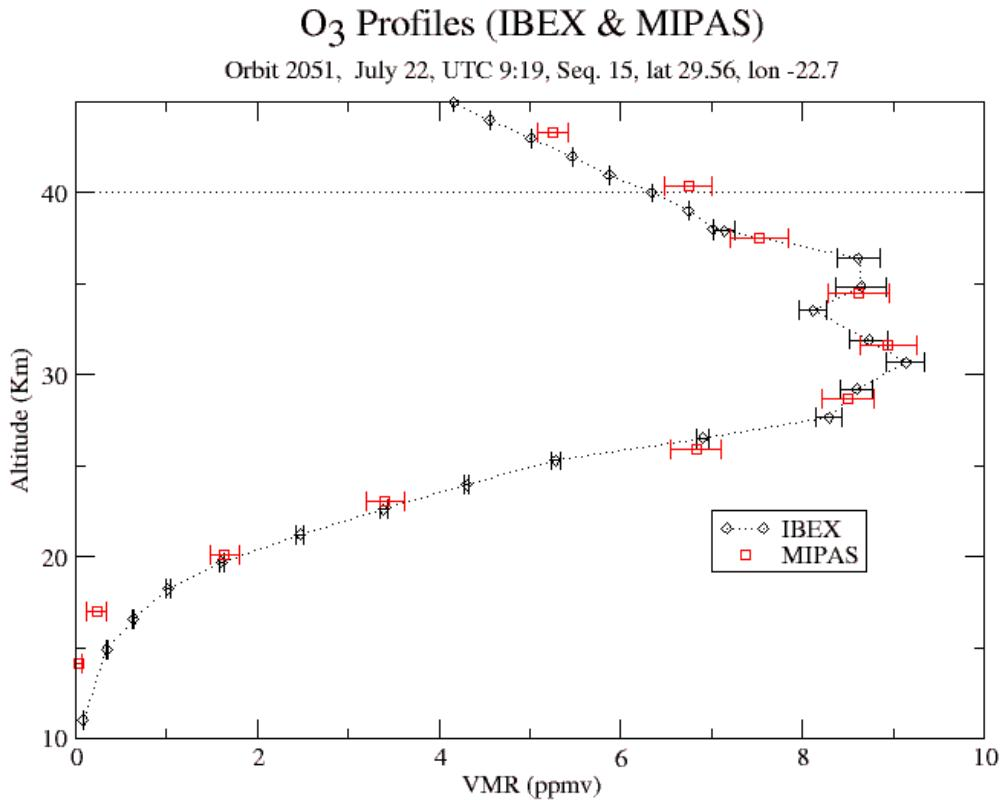
Fig. 7 Comparison of the average ozone profiles measured from balloon from Mipas
