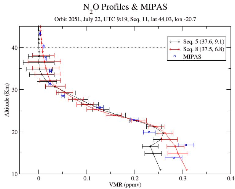
Fig. 8 – Profiles of  $\text{N}_2\text{O}$  measured from balloon and from Mipas
