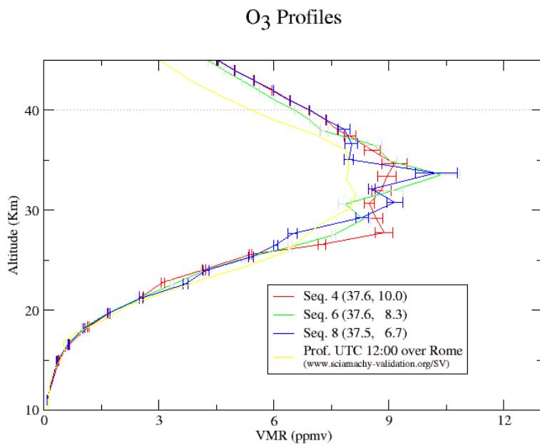
Fig. 6 O<sub>3</sub> profile for different sequences compared to on situ measurements
