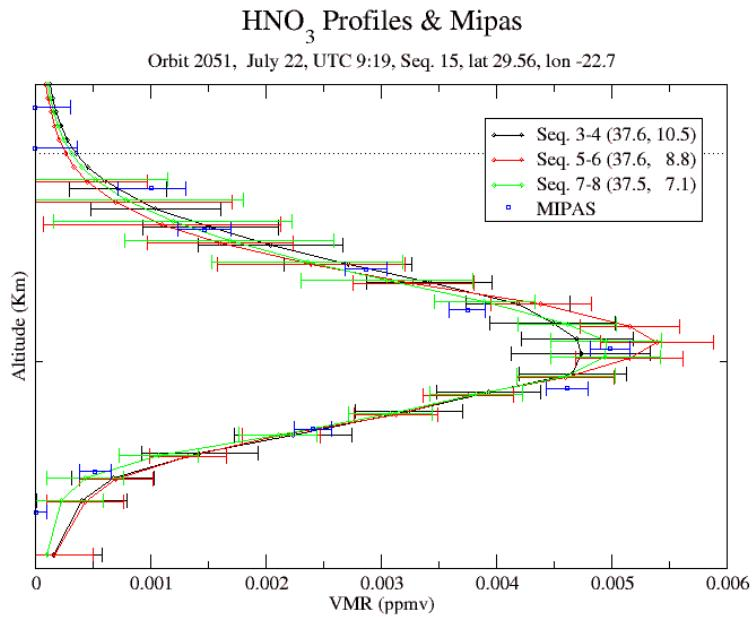
Fig. 9 – Profiles of  $\text{HNO}_3$  measured from balloon and from Mipas
